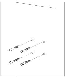
Step 3. Use the self-tapping screws (x4) to tighten the wall bracket to the preinstalled expansion screws in Step 5.
