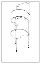
Step 4. Install the thermometer to the pre-installed wall bracket by tightening the big nut.
